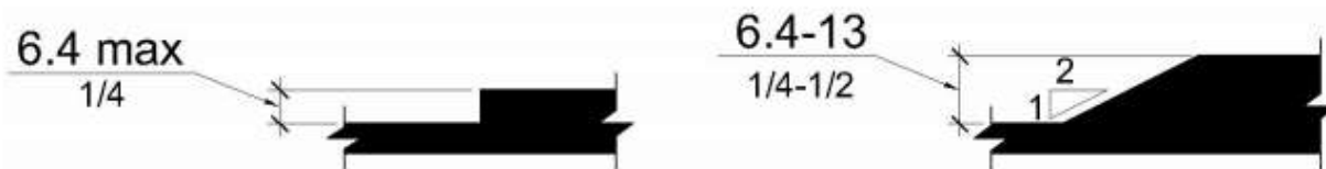
Figure 33 - Vertical surface discontinuities. On the left, a discontinuity of \frac{1}{4} in without a beveled edge. On the right, a discontinuity between \frac{1}{4} and \frac{1}{2} in., shown with the required 1:2 beveled edge.
